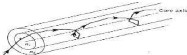
**14. Write the acceptance angle condition for the skew rays.**
