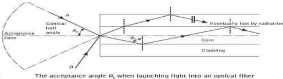
**11. A silica optical fiber with a large core diameter has a core refractive index of 1.5 and a cladding refractive index of 1.47. Determine the acceptance angle in air for the fiber.**
