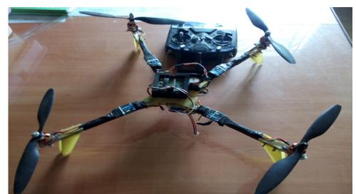
The Mini Drone is done by using wireless communication system. It has design to become an indispensable tool for the military. This project includes a camera and telemetry that will allow watching live video from the mini drone on a laptop that is located up to two miles away. The mini drone is controlled through graphical user interface. All signals from sensors are processed by Arduino Uno microcontroller.
